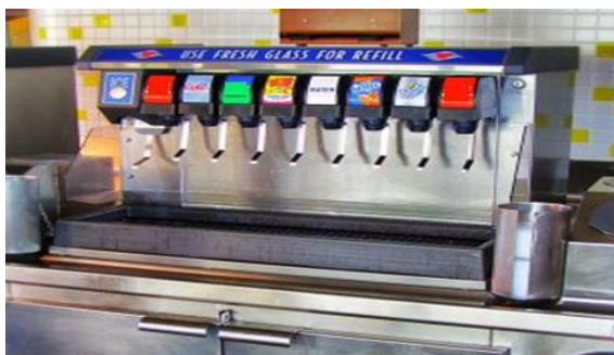
Equipment Sealed to Counter Top
